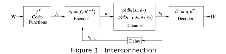
Choose encoder and decoder to transmit message over the channel to minimize the probability of error
